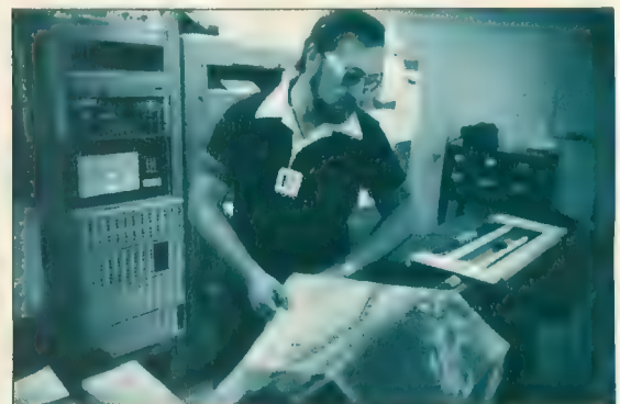
"Massaging" data: Bob Levno checks a weather facsimile map as it comes out of the plotter.
